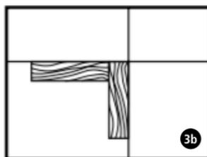
5. Install the second-floor board (tongue on the left) at a right angle with the first board (tongue on the right) to form an arrow-shaped pattern (illustration 4a and 4b) pointing in the right direction. The installation of all other floor boards will follow the same procedure.
